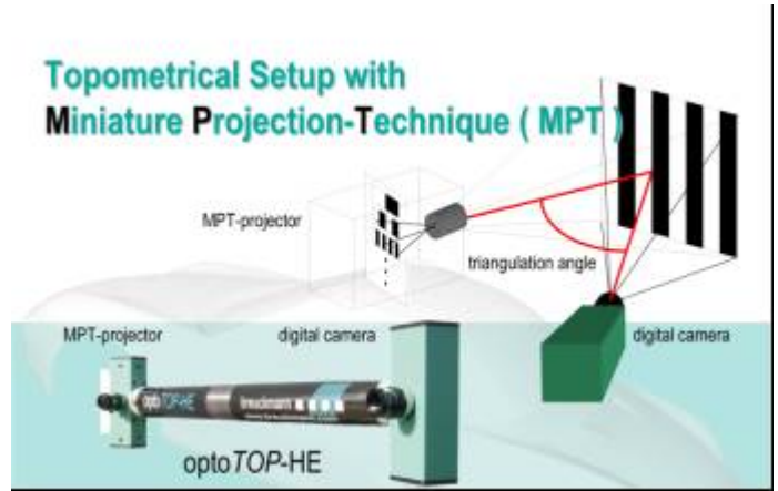
Fig. 8 Structured Light (triangulation) technique.
