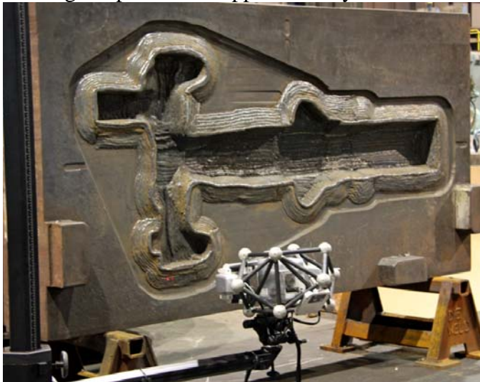
450°F Welded Die ready for scanning – Note red dot laser focusing pointers in front of scanner at edge of the weld.
