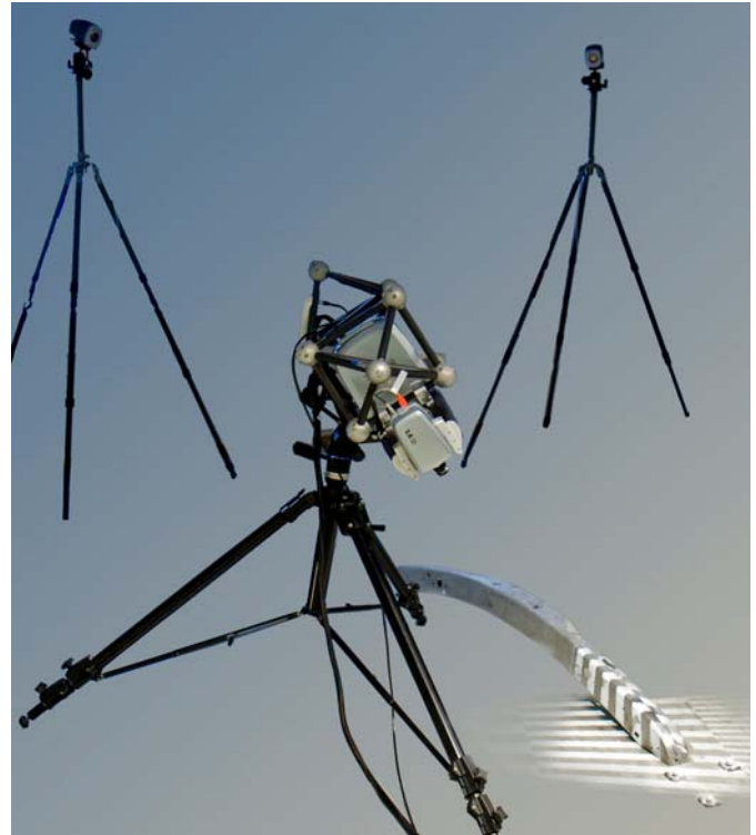
NaviSCAN3D System showing Metronor DUO cameras and Breuckmann StereoSCAN3D fitted with NaviTarget
