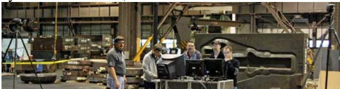
View of the NaviSCAN3D system, with curious onlookers Metronor DUO cameras are in upper left and right of photo & the scanner is behind the cart in front of the die.
