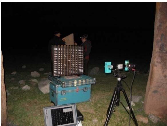
**Fig.11** System calibration (foreground) and cleaning monoliths (behind calibration plate) with bamboo skewers and toothbrushes to remove accretions [Bathow, 19 June 2007]
