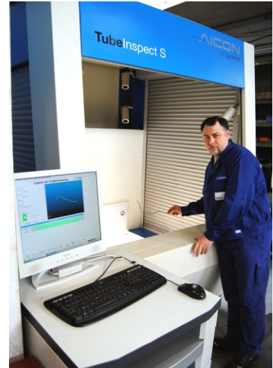
Valentin Medvedkins: “Thanks to TubeInspect, readjustment of our CNC bending machines is done instantly.”
