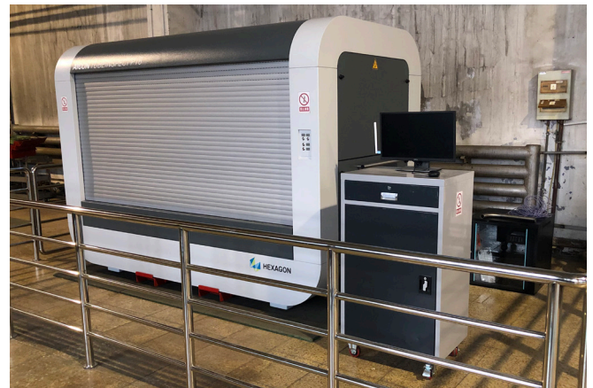
Thanks to its enclosed housing, TubelInspect is the perfect measuring system for the shop floor.
